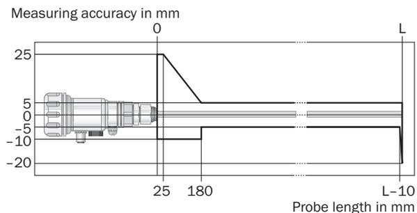
**Accuracy diagram without parameterized tank**
