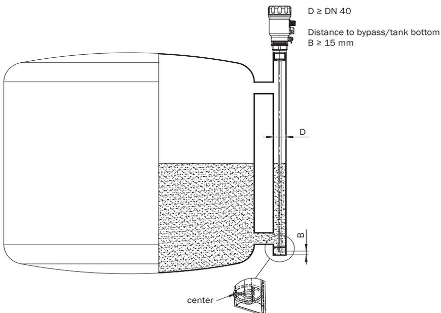
Centering: To prevent contact between the probe and the bypass pipe during oscillations, the probe should be centered according to its length and depending on the diameter of the bypass pipe. To do this, it is necessary to insert one or two centering pieces (see accessories). The use of LFP in bypass and immersion tube systems are not hygienic, because these systems are very difficult to clean.
