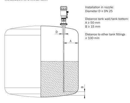
In a 3-A compliant installation, the neck height shouldn't be bigger than the neck diameter. Tank, pipe and process connection (tank side) should follow the guidelines and applicable standards for hygienic design such as roughness of wet parts Ra< =  $0.8 \mu m$ .
