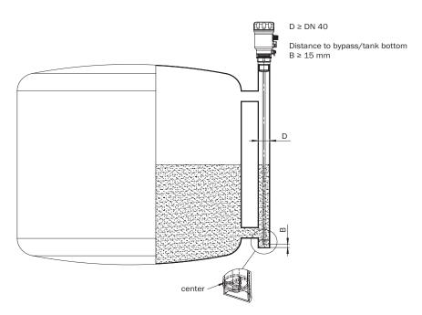
Centering: To prevent contact between the probe and the bypass pipe during oscillations, the probe should be centered according to its length and depending on the diameter of the bypass pipe. To do this, it is necessary to insert one or two centering pieces (see accessories). The use of LFP in bypass and immersion tube systems are not hygienic, because these systems are very difficult to clean.
