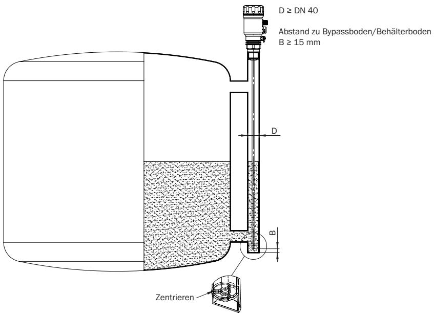
Centering: To prevent contact between the probe and the bypass pipe during oscillations, the probe should be centered according to its length and depending on the diameter of the bypass pipe. To do this, it is necessary to insert one or two centering pieces (see accessories).
